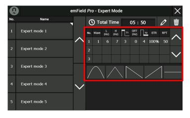
Choose the parameter to change. Wave, L (Hz), H (Hz), T1, Off, T2,, Strength, Repetition can be set in this mode by using the central control knob (6) which changes the parameter values.
