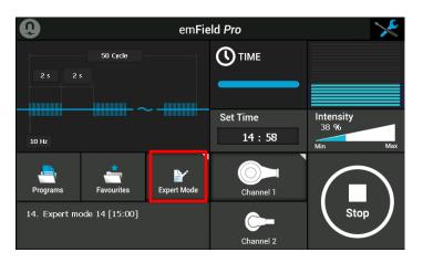
To change settings press Expert Mode on the touch screen for 2  $\sim$  3 seconds to set the parameter values.
