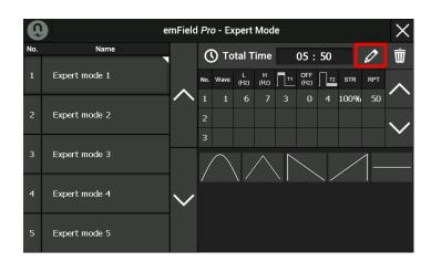
Each mode has 9 sub-modes with different parameter sets. The Expert mode operates sequentially from sub mode 1.
